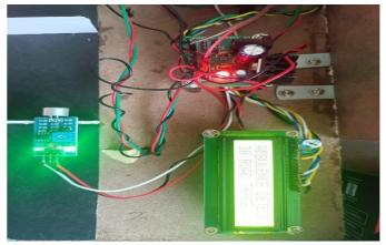
When an ambulance is being detected it is being displayed in the LCD with the indication on which road the ambulance or emergency vehicle is being detected.
