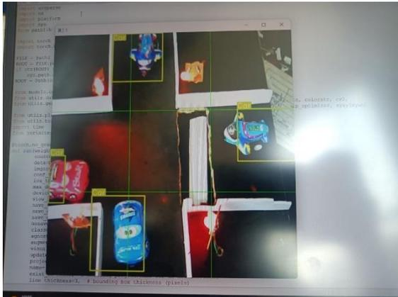
The car on each road is being detected and a pedestrian safety hump is being used which will be raised whenever the pedestrian will be crossing the road i.e. whenever the red light is being displayed. This we ensure that accident is prevented and pedestrian is also safe.
