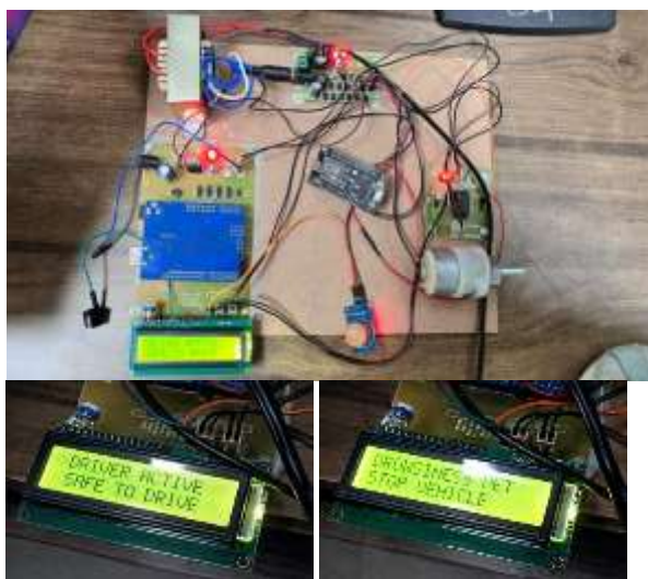
Fig-9: Hardware kit showing output of driver state
