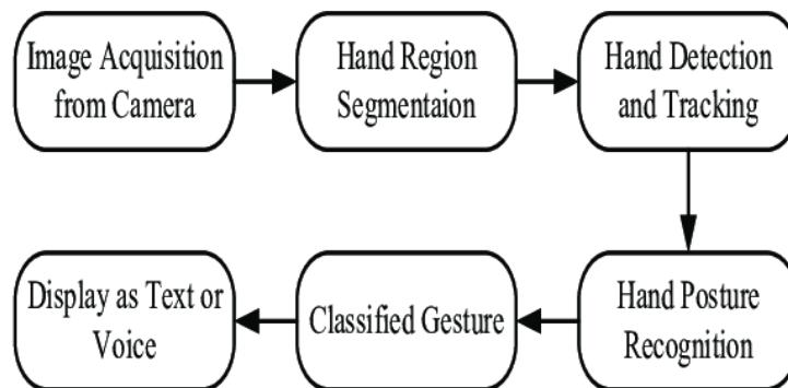
Fig. 1: Block diagram for gesture System
