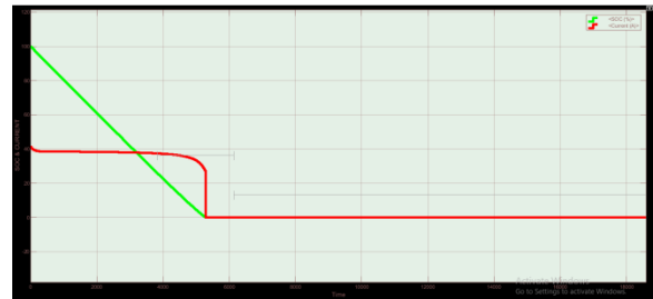
Figure 12.4:- SOC & CURRENT WAVEFORM OF DISCHARGE OF PARALLEL CONNECTED LITHIUM ION-LITHIUM ION BATTERY WITH LOAD AS STEP SIGNAL FOR 6 HOURS
