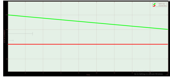
Figure 12.2:- SOC & CURRENT WAVEFORM OF DISCHARGE OF PARALLEL CONNECTED LITHIUM ION-LITHIUM ION BATTERY WITH LOAD AS 72 OHMS FOR 500 HOURS
