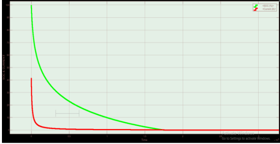
Figure 12.6:- SOC & CURRENT WAVEFORM OF DISCHARGE OF PARALLEL CONNECTED LITHIUM ION-LITHIUM ION BATTERY WITH LOAD AS STEP SIGNAL WITH RAMP START FOR 80 HOURS
