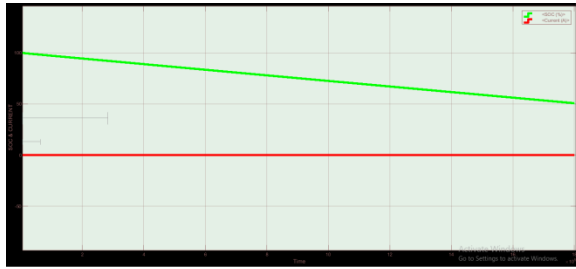
Figure 4.2:- SOC & CURRENT WAVEFORM OF DISCHARGE OF PARALLEL CONNECTED LITHIUM ION-LITHIUM ION BATTERY WITH LOAD RESISTANCE OF 72 OHMS FOR 500 HOURS
