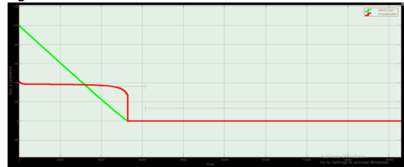
Figure4.7:- SOC & CURRENT WAVEFORM OF DISCHARGE OF PARALLEL CONNECTED LITHIUM ION-LITHIUM ION BATTERY WITH LOAD AS STEP SIGNAL FOR 6 HOURS
