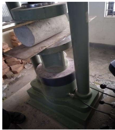
Fig. 9. Flexural Strength Test for Concrete Cylinder
