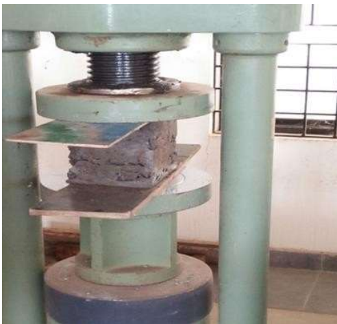
Fig. 7. Compressive Strength Test of Concrete Cube
