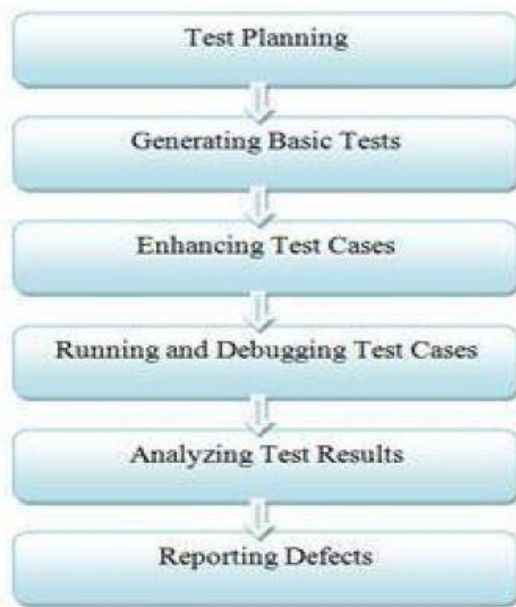
Figure 3.1: Selenium Testing Process
