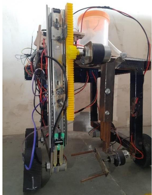
Figure 4.4 Prototype view of rack and pinion
