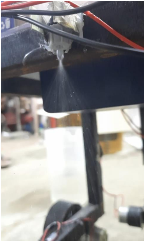
Figure 5.1 water spraying from nozzle testing
