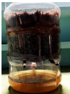
Fig 8: Filtration with coarse aggregate, well graded soil and coconut coir
