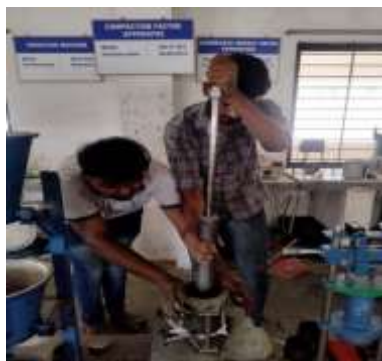
Fig 3.16 Placing the mix & compacting
