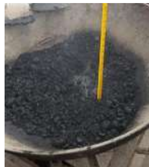
Fig 3.15 Marshall Mix preparation
