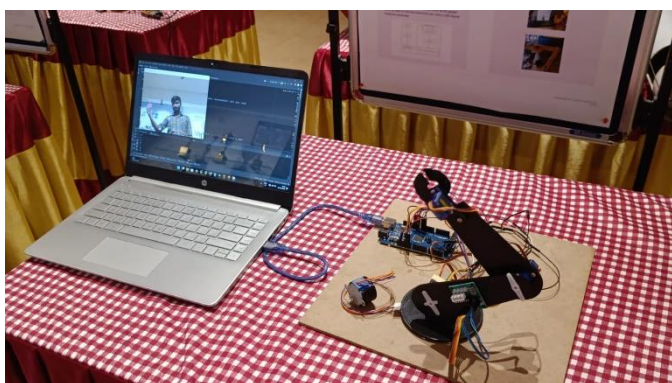
Figure 5: 3D printed complete arm in action.
