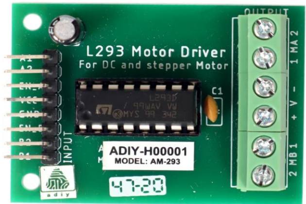
Fig-4: Motor Drive
