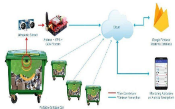
Fig 3: Waste Management Using IoT
