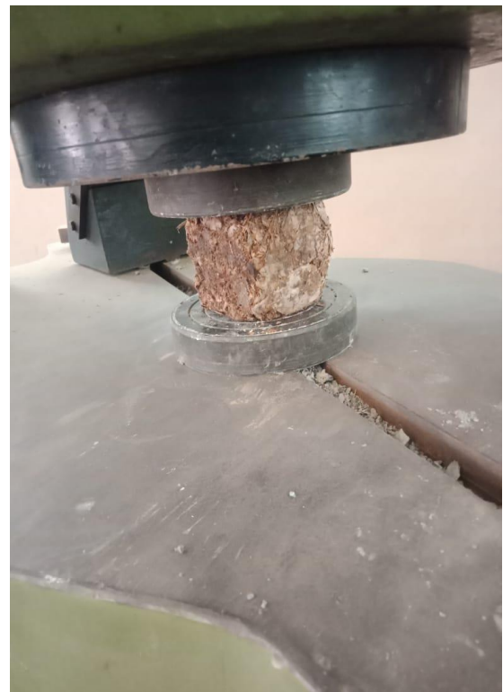
Fig 3: Checking Compressive strength of briquette on UTM machine
