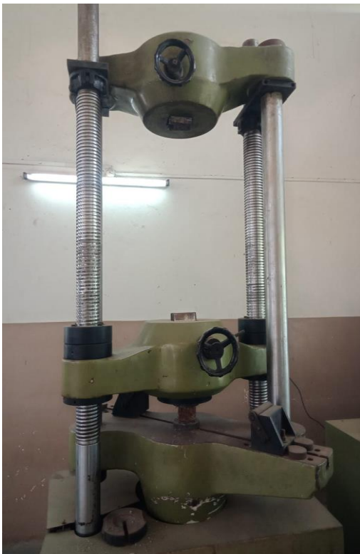
Fig 3: Checking Compressive strength of briquette on UTM machine
