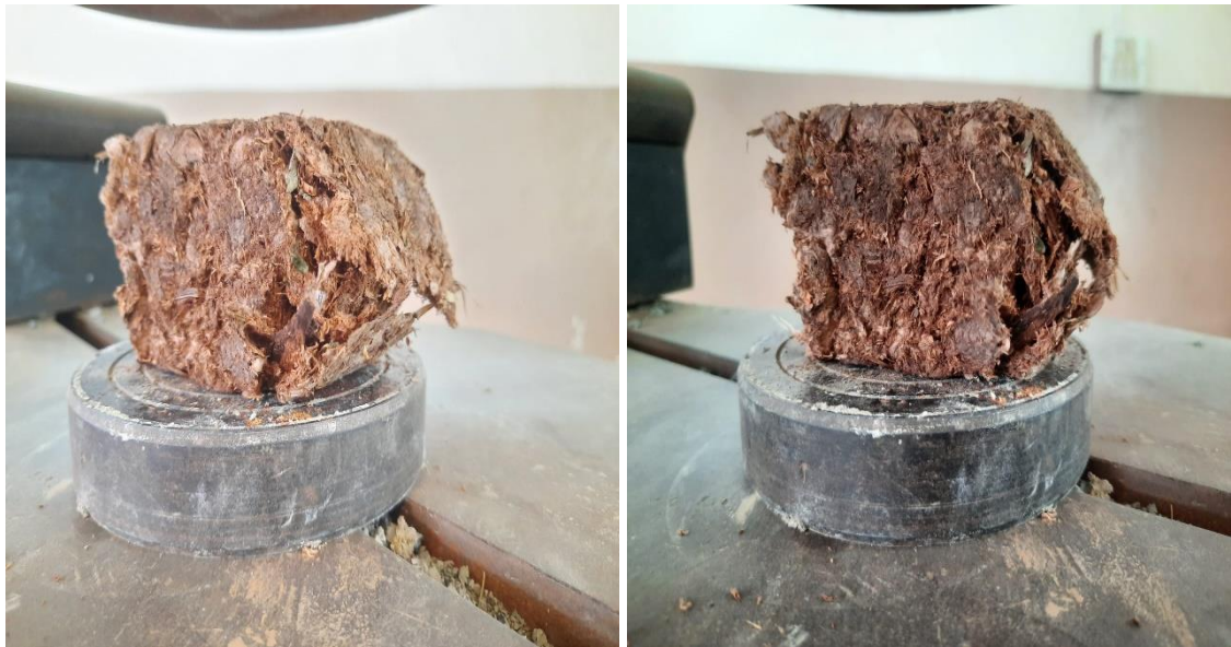
Fig 4: Briquette after applying the load
