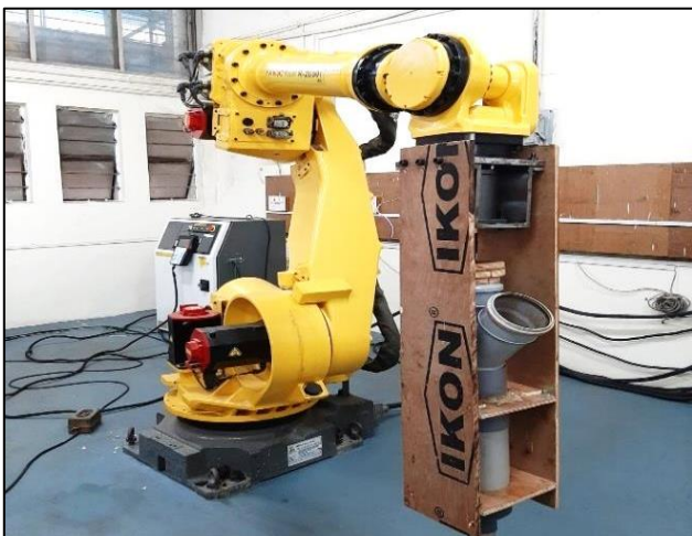
Fig.4 Extruder setup on Fanuc r2000 i165
