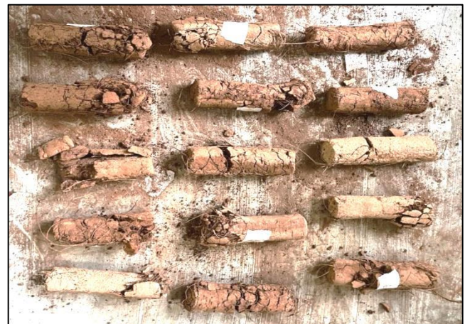
Fig.5 Tested soil specimens on UCT
