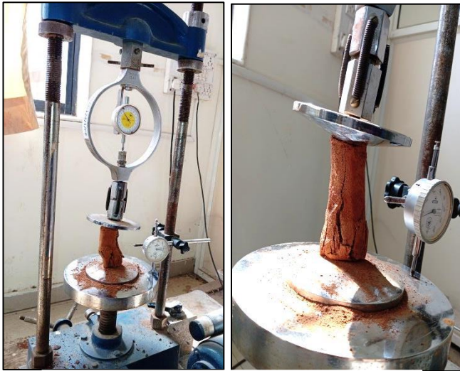
Fig.1 Testing of soil specimen on UCT setup
